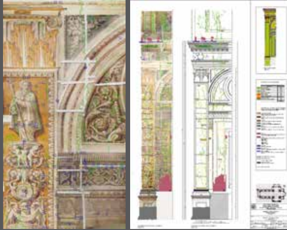
St. Andrew's Basilica in Mantua: decay mapping in the pilot-yard (Photo and drawing D. Del Curto)
