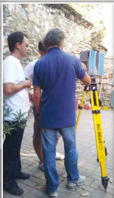
First external station of 3D laser scanner survey
