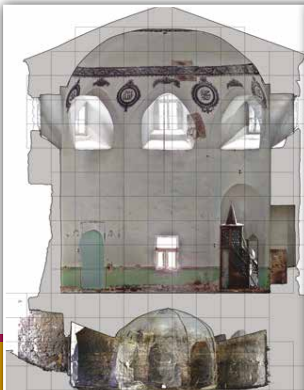
2D drawing table with CAD section and planar point cloud image
