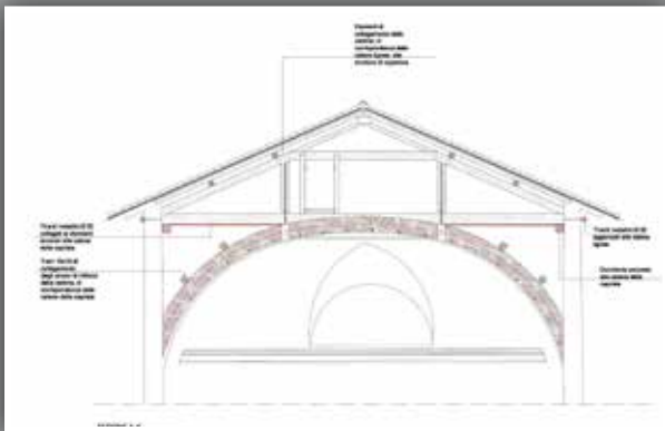
Detail of the reinforcement of the ceiling
