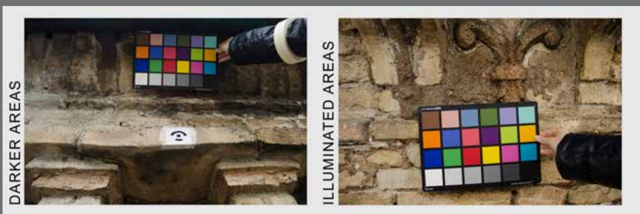
Colour checker positioned in different areas of the cornice in order to provide proper calibration of areas characterized by different illumination.
