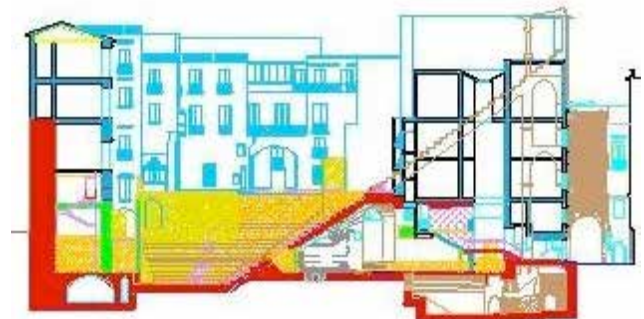
Section on the cavea, the ambulatory and substructures up to the “Anticaglia arch”
