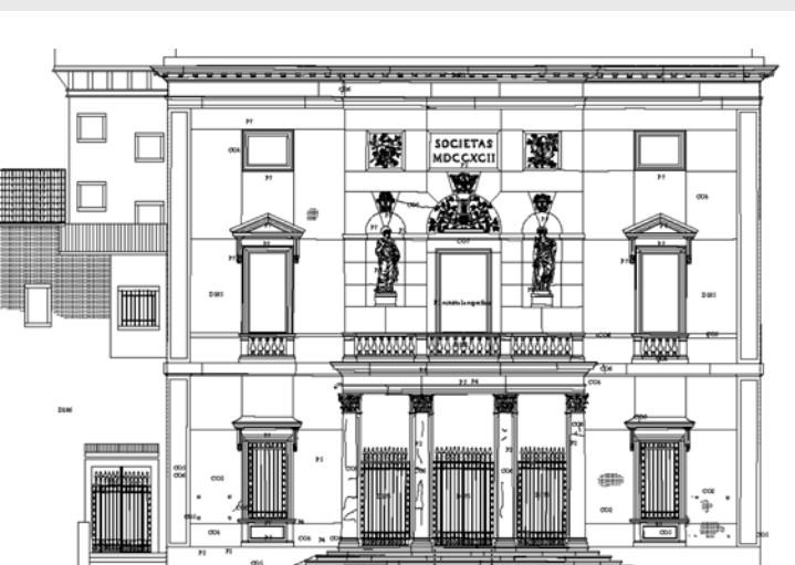
Fig 4. Detailed drawing with single marble slabs related to a fixed price contract with detailed descriptions of complete restoration works
