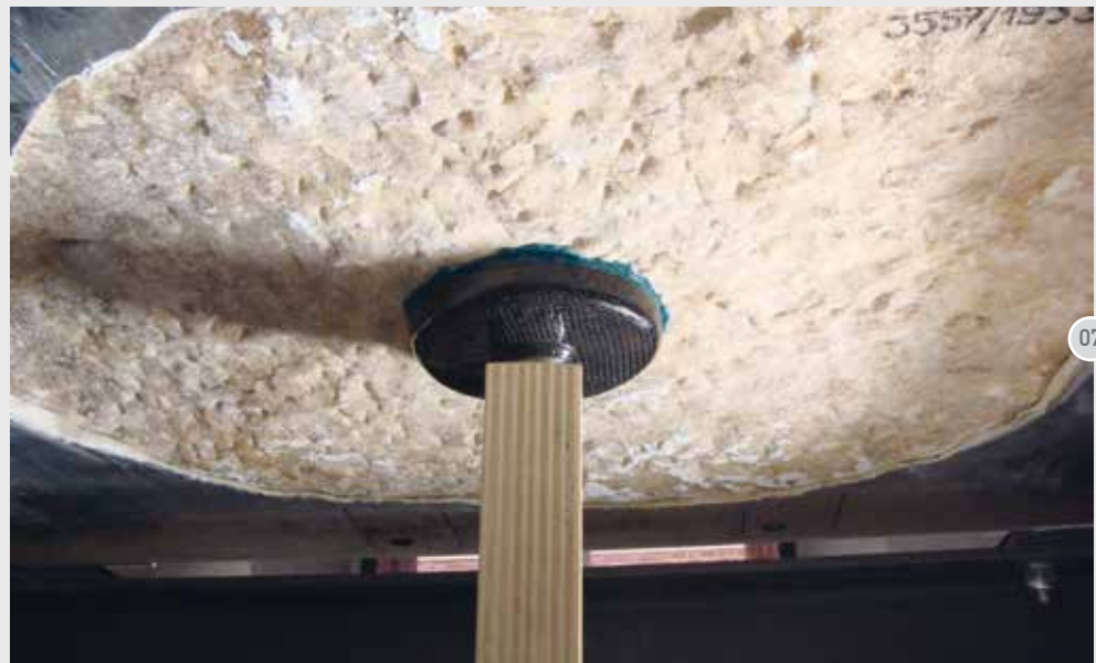
Fig 7. Bonding of Kimitech FRP-LOCK PR
