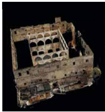
Fig 2. Tri-dimensional cloud of points and graphic rendering of North Elevation
