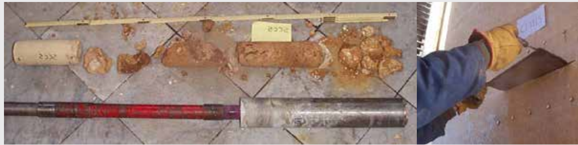
MDT: core drilling and flat jacks
