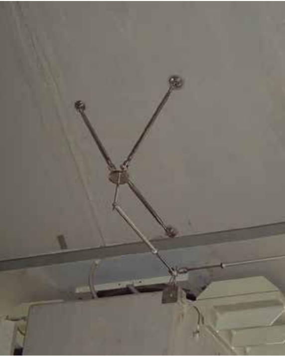
Static Data Logging system: Displacement Transducers with customised holding device. Temperature and Relative Humidity Indoor Sensors
